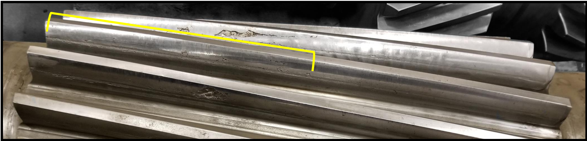
Wear shifted to the left side of the tooth width
