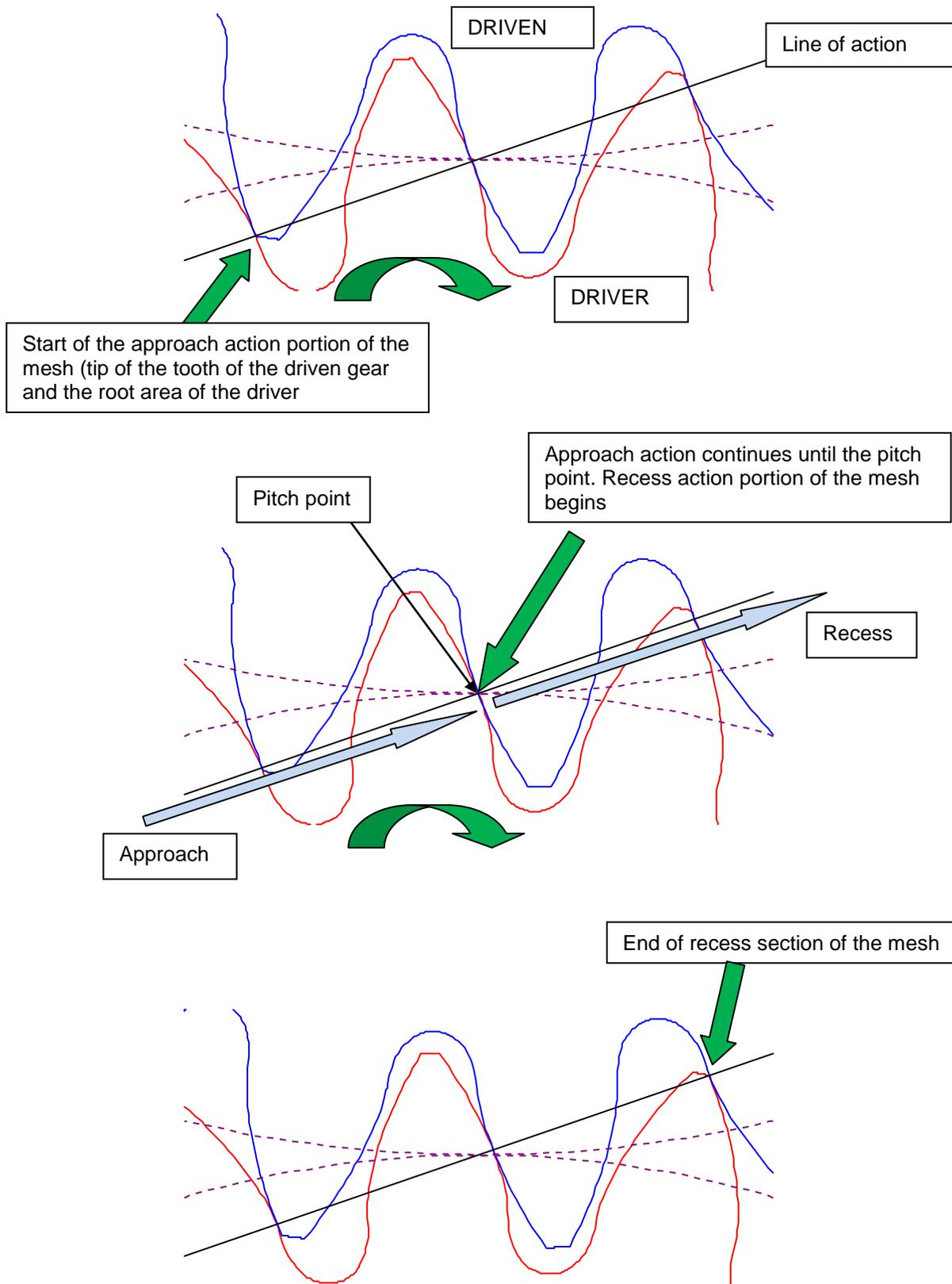
Generally, it's desirable to modify tooth proportions in order to decrease the negative effects associated with approach and promote the involute action during recess. Depending on the design requirements and other constraints, multiple solutions can be achieved based on the approach taken:
